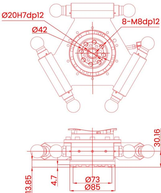
**基座安装 Base installation (mm)**
