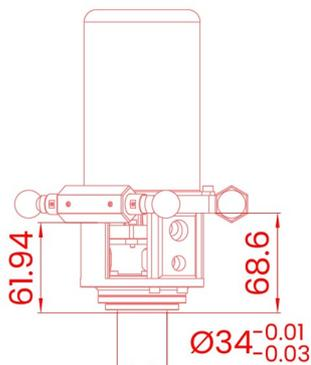
基座安装 Base installation (mm)
