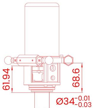
基座安装 Base installation (mm)
