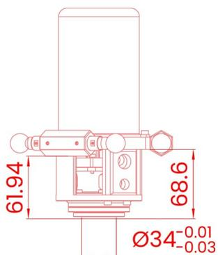
基座安装 Base installation (mm)
