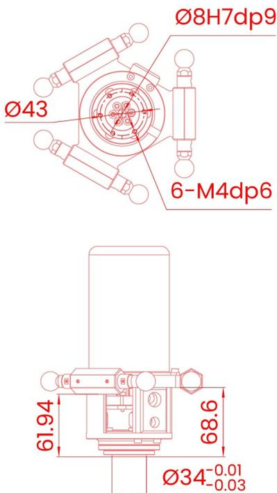
基座安装 Base installation (mm)
