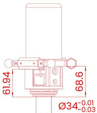
基座安装 Base installation (mm)
