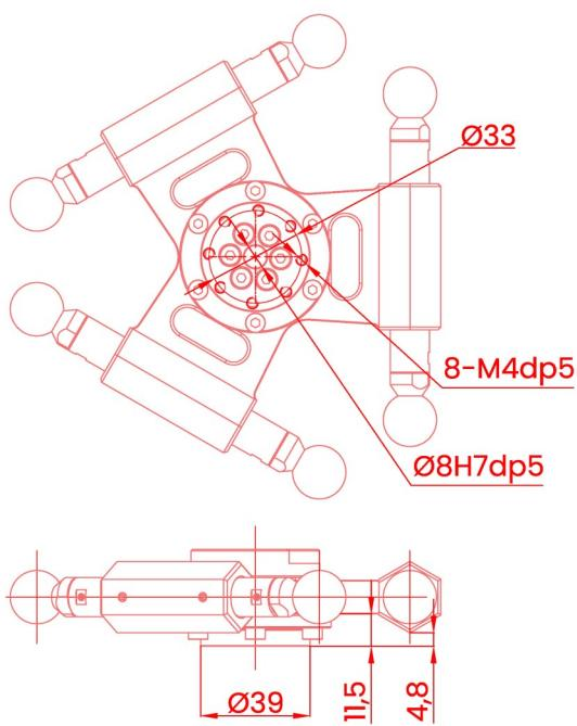
基座安装 Base installation (mm)
