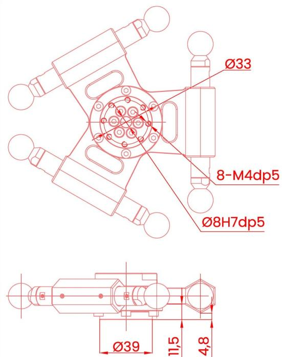
**基座安装 Base installation (mm)**
