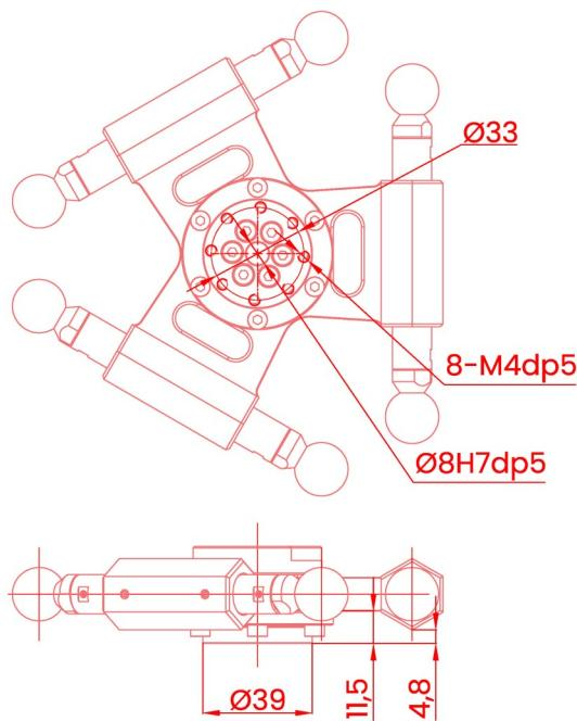
基座安装 Base installation (mm)
