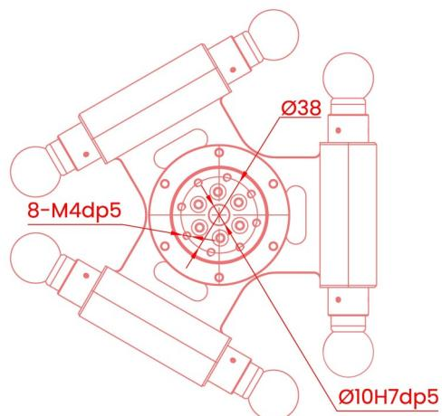
基座安装 Base installation (mm)
