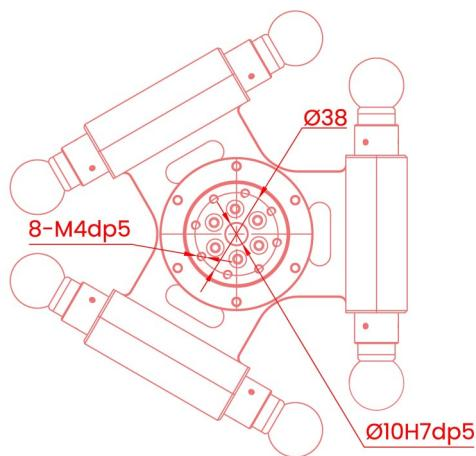
基座安装 Base installation (mm)
