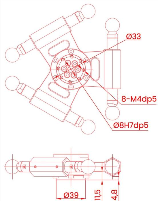
基座安装 Base installation (mm)
