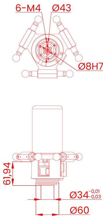
基座安装 Base installation (mm)
