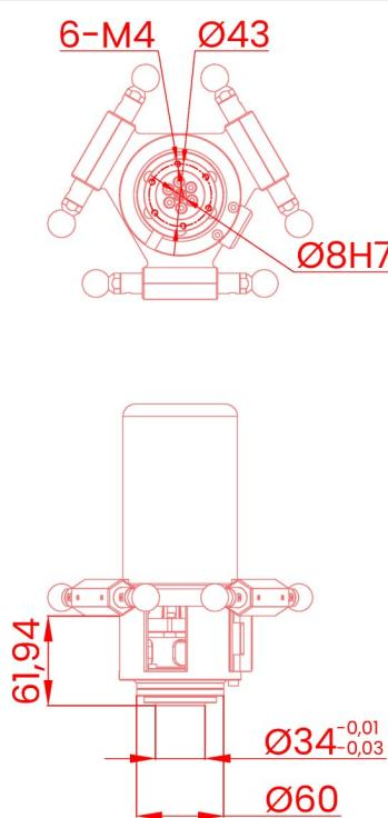
基座安装 Base installation (mm)
