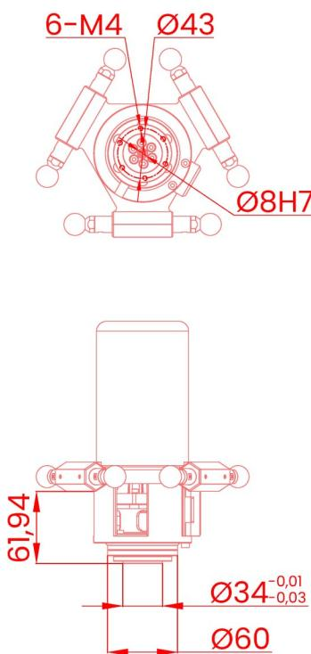
**基座安装 Base installation (mm)**
