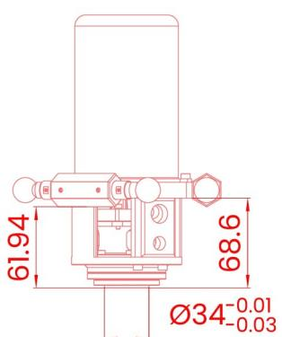
基座安装 Base installation (mm)
