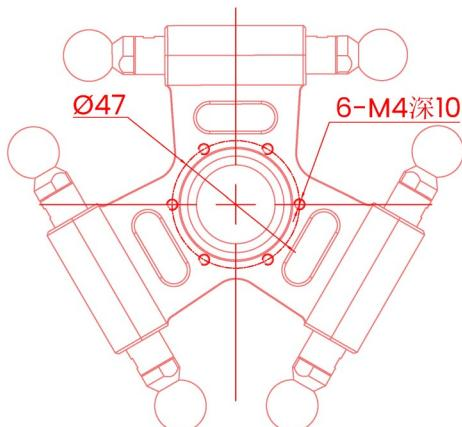
基座安装 Base installation (mm)
