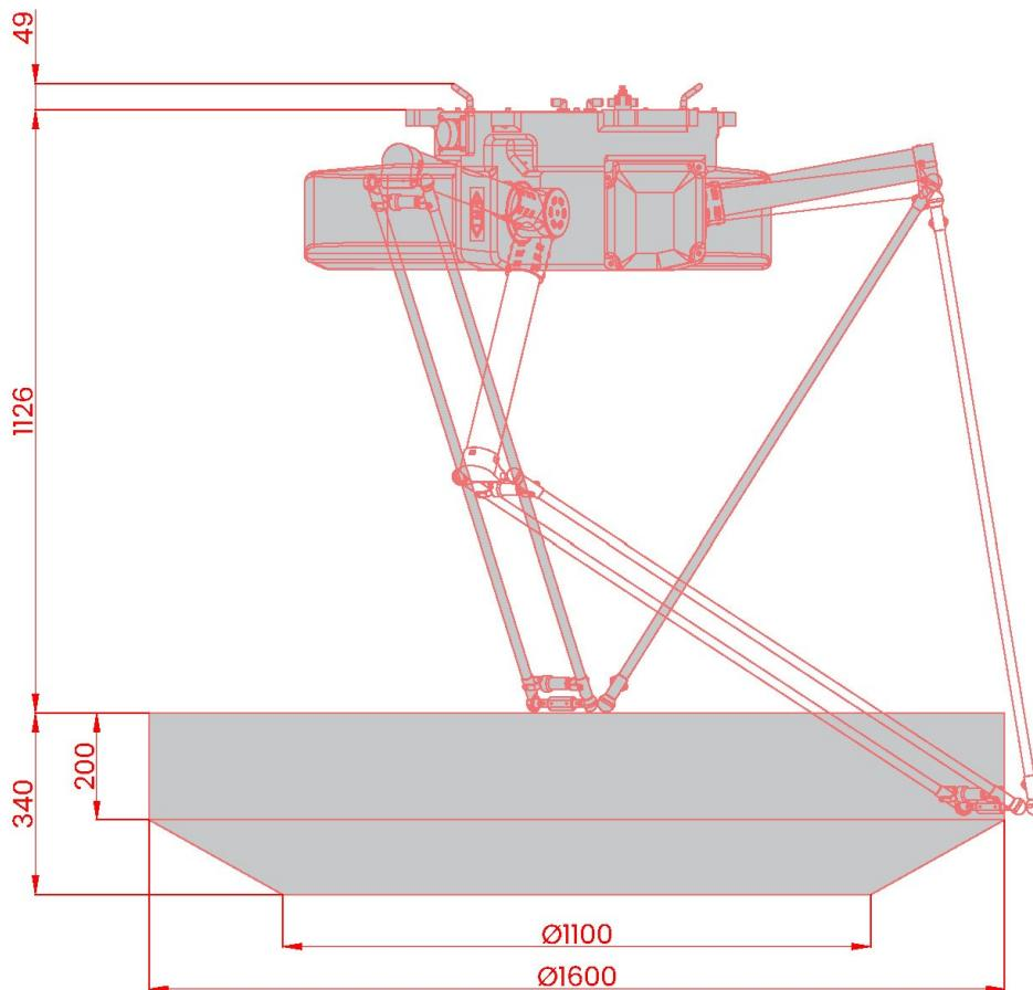
**法兰 Flange (mm)**
